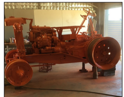
The tractor stripped, rebuilt and in the stage of being repainted the distinctive Chamberlain orange
